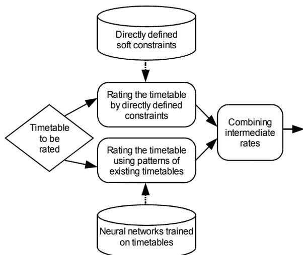
Figure 3. The timetable-rating block as a part of genetic algorithm
