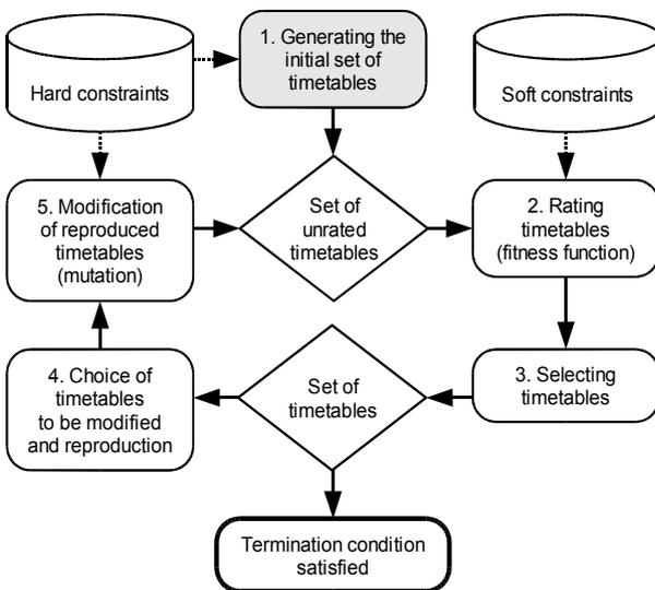
Figure 2. The schema for genetic algorithms in timetabling
