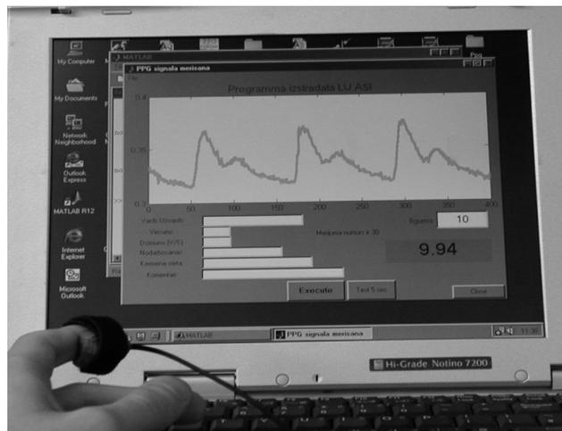
Fig. 1. Portable version of single-channel PPG sensor: application for the fingertip monitoring.
