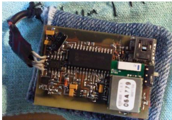
Fig. 2. Outlook of the wireless PPG sensor device (dimensions 45x30x7mm).
